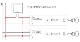
Remarks: use only open push switch (without indicator light). When using synchronous connection, the line length between each device and equipment shall not exceed 20 meters.
